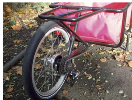
● (Above) The 8Freight's hubs are supported on one side only. Puncture repairs are easy, upgrades less so (Below) The rear rack makes it easier to secure oversize loads that overhang the main luggage platform
