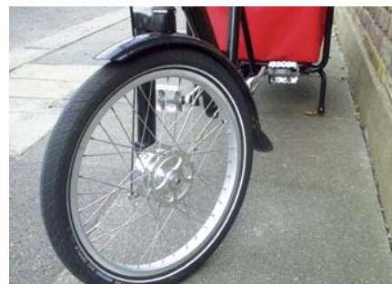
● (Above) The 8Freight's hubs are supported on one side only. Puncture repairs are easy, upgrades less so (Below) The rear rack makes it easier to secure oversize loads that overhang the main luggage platform
