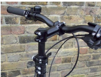
● (Above) The Bullitt's front load platform is easy to keep an eye on. Steering is via a rod to the fork (Below) The Bullitt's 'easy up' stem gives 100mm of instant handlebar-height adjustment
