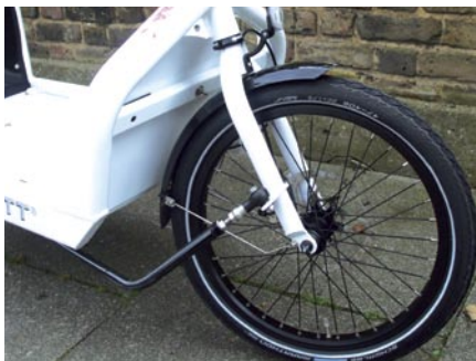
● (Above) The Bullitt's front load platform is easy to keep an eye on. Steering is via a rod to the fork (Below) The Bullitt's 'easy up' stem gives 100mm of instant handlebar-height adjustment
