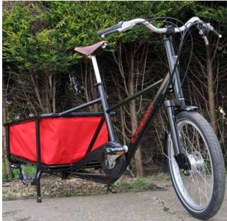
ABOVE: The essential chainguard and twin leg stand that always secured our loaded bike.
