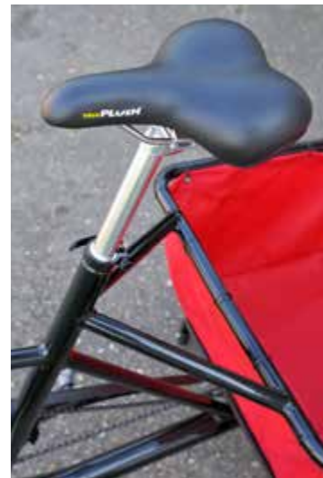
BELOW: Velo Plush saddle is standard. The new frame benefits from a triangulating central frame member.
