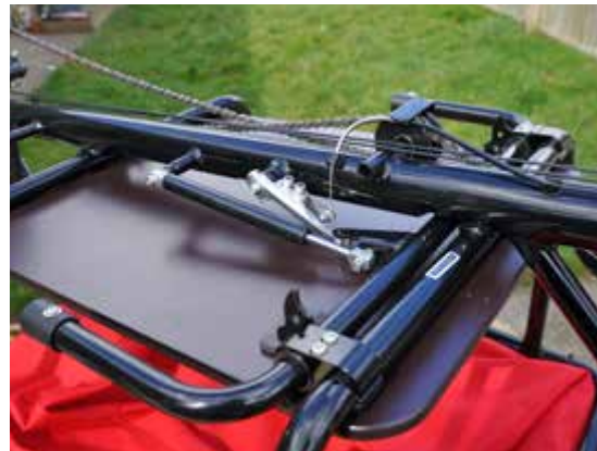
ABOVE: Underside view of the cable-operated stand release.
