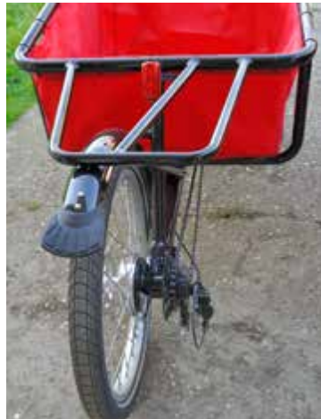
ABOVE: The essential chainguard and twin leg stand that always secured our loaded bike.
